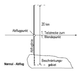
**Start line type 2**: 10 minutes before crossing start line pilot has to set a marker in the IGC-file. The start is valid when the start line is crossed 10 minutes after declaration +/- 1 minute. A new start declaration marker can be set when the preceding 10 minutes interval has ended.
